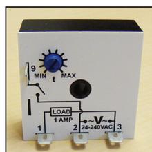
**Built-in Time Delay Relay-** Provides a delay for shutting off the air curtain after the door closes. This is useful for doors that see a lot of foot traffic, so that the unit is not constantly turning on and off. This timer is factory set at 30 seconds but is adjustable up to 100 seconds.
