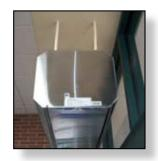
TOP MOUNT -- Unit has four 3/8-16 threaded inserts for installing one end of threaded rods. The other ends of the threaded rods can be attached to the ceiling. Threaded rod should not extend more than 3/4 inch into air curtain.
