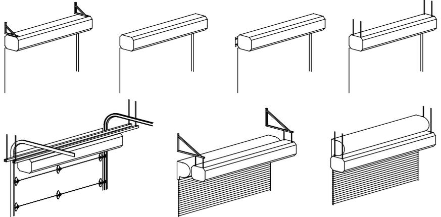
Note: All hardware and brackets must be of sufficient strength to safely support air curtain.
