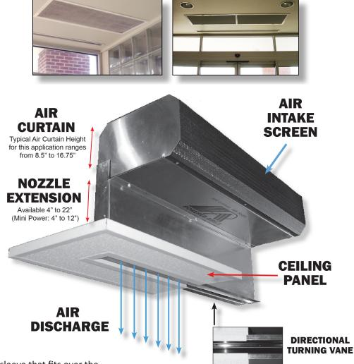
The top of the extension is like a sleeve that fits over the discharge of the air curtain. It is attached to the air curtain using self tapping screws fastened to the case of the unit.
