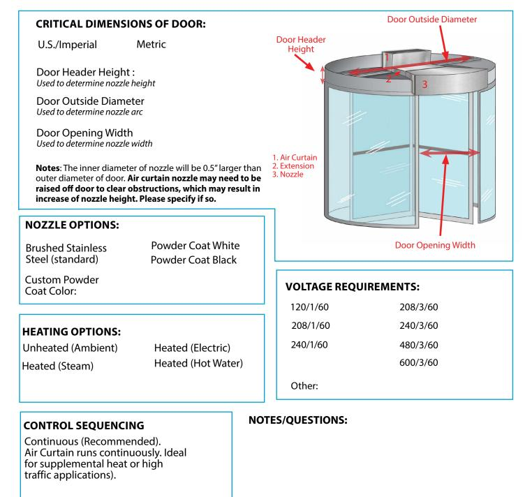
Dry Contacts (air curtain activates with dry contacts in door or motion detector (not supplied).
