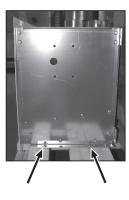
The air curtain has rear flanges with six holes for ½ inch bolts which are used to lag the unit to the bottom of the crate frame. Unscrew to remove air curtain. For convenience, these same holes can used if mounting the air curtain directly to the wall.
