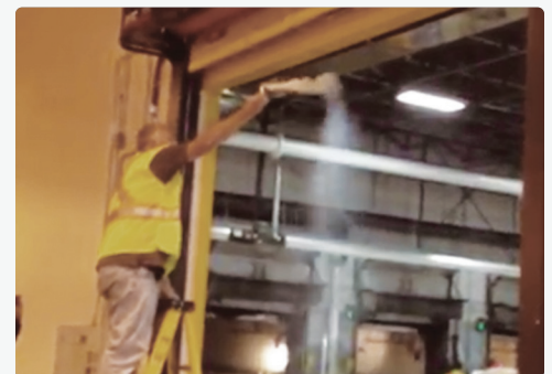
With the air curtain operating, the discharge of air forms a thermal barrier that deflects the smoke and prevents infiltration.
